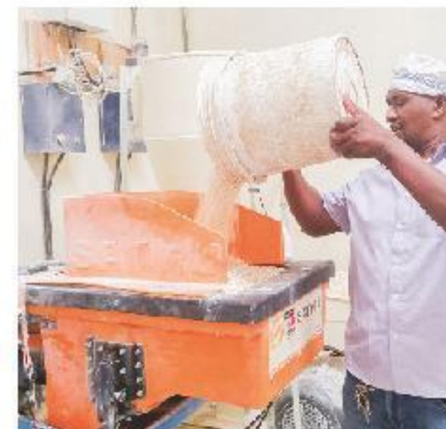
Loading maize onto the Dosifier for fortification. NELSON MWANGI | SANKU
